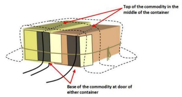
4.2.5 Three or more containers under a gas-proof sheet is a single enclosure and must have at least one sampling tube placed as close as practicable to the top of the commodity in the middle of each container (Figure 3).
