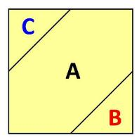
A Standard concentration. B Minimum concentration to allow top-up. C Maximum top-up concentration. See <u>Appendix 4: Methyl bromide monitoring table</u>. Note: (C – lowest concentration reading) x enclosure volume = top-up amount.
