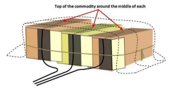
Four containers in one enclosure must have at least four sampling tubes, five containers, five sampling tubes and so on.
